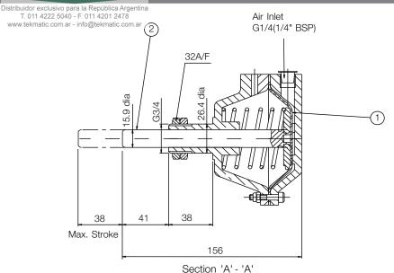
This range of pneumatically operated brakes uses dry and filtered compressed air at pressures up ot 7 bar. Pneumatic brakes require a control valve which may be operated either manually, or by pneumatic or electrical signal.
